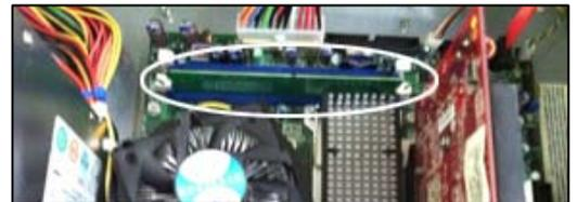
7. Push down on the two white or beige thumb latches securing the DIMM on either side. Make sure the latches are pushed outward to the open position. **You must remove any and all DIMM before moving to Step 8.**
