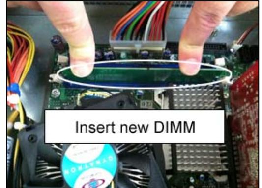
10. Insert the bottom edge of the DIMM into the socket. Push down on the top edge of the DIMM until the retaining thumb latches snap into place. **Do not force the DIMM into the slot.** Make sure the latches are firmly in place.
