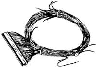
1. If you are installing BIG BUCK HUNTER CALL OF THE WILD into a cabinet with a pre-installed JAMMA harness, it may not have a wire for the test switch. You will have to add a contact to the edge connector at the proper position (position 15). Some cabinets
