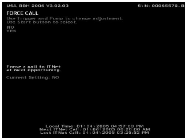
**FORCE CALL** menu can be used to make your machine manually call ITNet at a time other than its regularly scheduled hour. This can be used when you are trying to fix the modem or phone line on your machine, or if you are about to disable calling and want the last set of information to be transmitted to the ITNet servers. This setting defaults to NO. If you select YES, as soon as you exit all of the menus the machine will automatically attempt to call ITNet.
