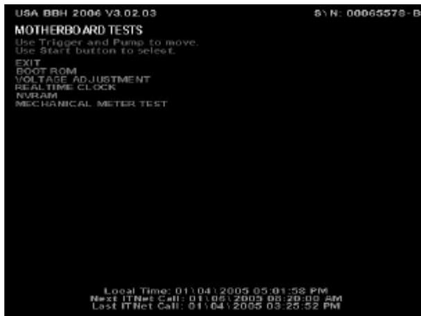
**BOOT ROM** tests the memory your game boots from. To activate this test press the START button. You will get one of two messages: “BOOT ROM CHECKSUM IS CORRECT” or “BOOT ROM CHECKSUM IS INCORRECT”. If you get the failure message please contact your local distributor or the IT Service Department.
