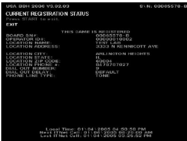
**CURRENT REGISTRATION STATUS** displays the ITNet information the machine is currently operating under. This will display the most current entered information, including the board serial number, your operator ID number, the location name, address, phone number, and the modem dialing instructions.
