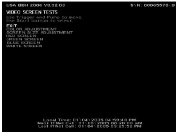
Exit these tests by pressing the START button. The screens help you test the condition of the monitor's components. Use these screens while adjusting your monitor so it looks as good as possible.
