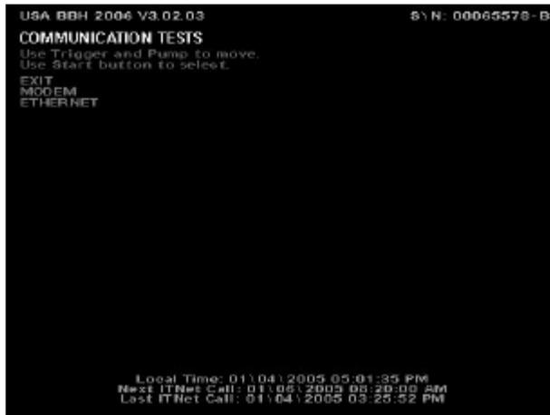
**MODEM** tests the existence of the modem as well as its ability to respond. Each machine needs its own working modem, even if daisy chained. Pressing the START button when MODEM is selected will activate the test and a pass or fail message will appear. If the modem test fails, contact your distributor or the IT Service Department.
