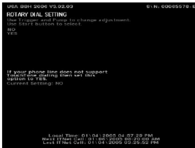
**ROTARY DIAL PHONE LINE** is the last of the quick ITNet/phone related menu functions you can access on this menu. While most phones use tone dialing, some still use rotary or pulse to dial. Accidentally setting this feature to YES on a tone line should not affect the call to ITNet.
