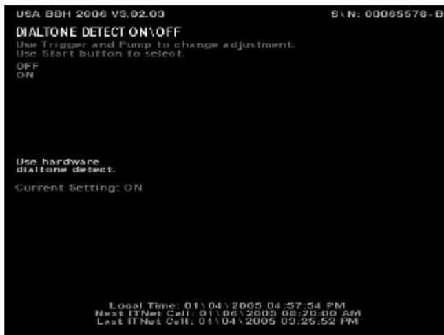
**DIALTONE DETECT** allows you to tell your machine whether or not to detect a dial tone when making an outside call. When set to ON, the machine's modem will wait to detect a dial tone before dialing. When set to OFF, the machine will not wait for a dial tone before dialing. For US machines, the default setting is ON and in most cases should not be changed.
