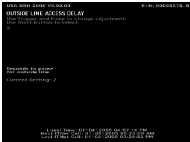
**OUTSIDE LINE ACCESS DELAY** is another quick access menu designed to help ensure calls get made successfully to ITNet. The number (2 is the default) you set here is the pause it uses to wait for the outside line. This is normally only required when you use a number to dial out with first, but won't hurt the machine if you leave the default set to 2.
