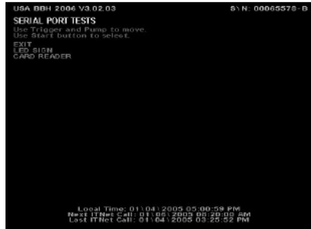
**LED SIGN** tests the integrity of the connection from the game to the LED sign and LED hardware. Press the START button to activate the sign test. The video screen will display the communication status. The LED sign will display the code version number, followed by a string of letters and numbers, then a solid bar will scroll across the display. Use this test to visually check for non-functioning LED segments. Press the START button to exit out of this test.
