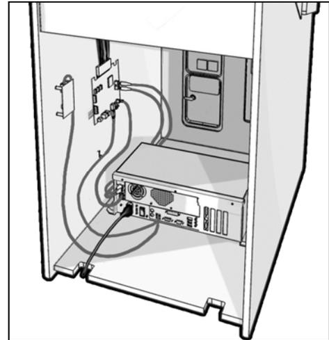
**Disconnect all I/O Board USB cables before transport.**
