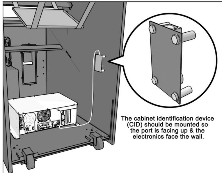
The cabinet identification device (CID) should be mounted so the port is facing up & the electronics face the wall.
