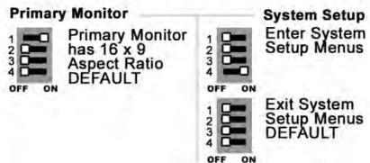
Note: In the Additional Settings above, ONLY the ON switch matters for correct setup and operation.
