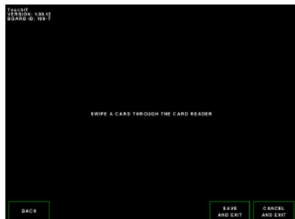
Swipe a card through the card reader. Normally the message “A CARD SWIPE HAS BEEN DETECTED.” is displayed, as well as the recognized card type. If you do not get the message, try swiping a card at different speeds or use a different operator or player card. If still unsuccessful, contact your distributor or the IT service department.
