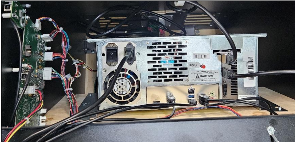
Final Connections with System Box Installed
