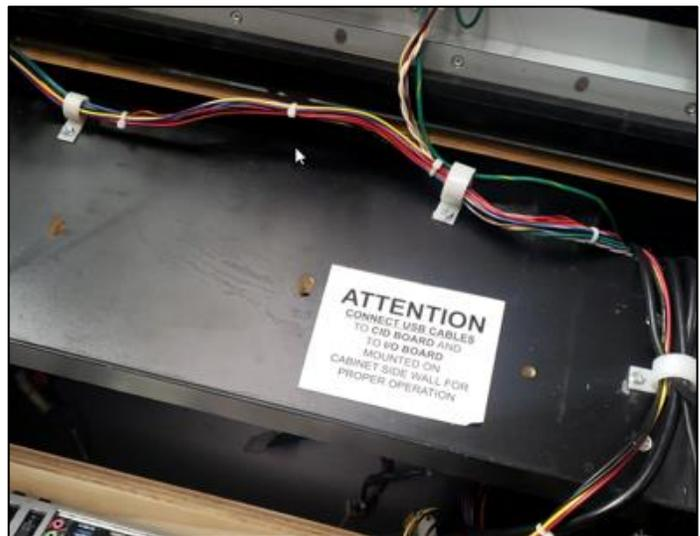
5. Remove Main Cable Harness from cabinet, coil and set aside. It will no longer be needed.
